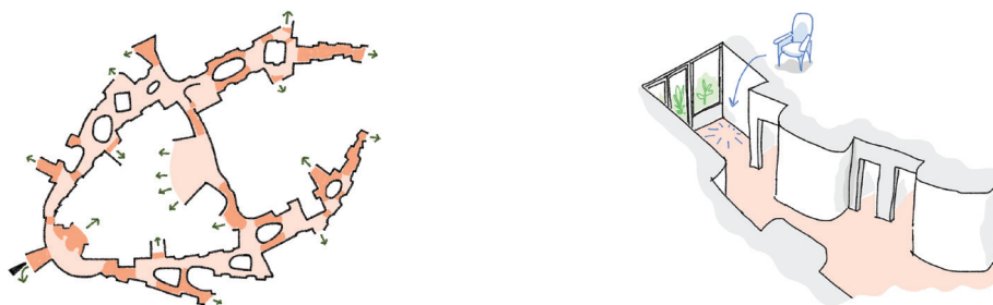
Figure 11: Floor plan of the Orb Pavilion walkways, highlighting viewpoints, direct exterior access (arrows), areas of constriction (dark), and expansion (light). Spatial dynamics continuously transform through interplays of openings, lighting variations, and bottlenecks. Source: (Marie Tesson 2024). Figure 12: Perspective view of an alcove in the Orb Pavilion, furnished and nestled within undulating walls, creating a secluded environment where the walkway contracts, marking the culmination of the building. Source: (Marie Tesson 2024)
