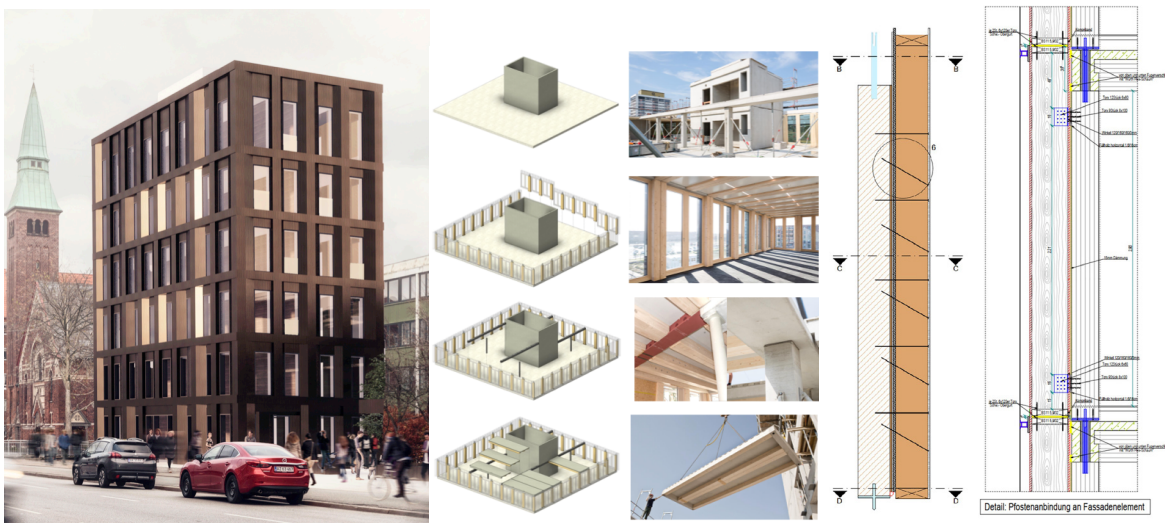
Figure 6, 7 and 8: Fig. 6 Visualisation of the student housing and café on Østerbrogade 190. Source (Vilhelm Lauritzen Architects, CREE Building 2018) Fig. 7: Detail that shows the montage of the façade elements, glulam beams and hybrid floor slabs. Source: (CREE Building 2018) Fig. 8: Two vertical sections construction drawings (to the left); the first showing the connection type using long screws. Source: (CREE Building 2018)
