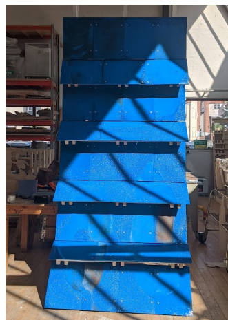
Figure 5: Polycarbonate panel assembly – façade - showing collage of imperfection characteristics created by top plate pressure applications. Source: (Author 2022)
