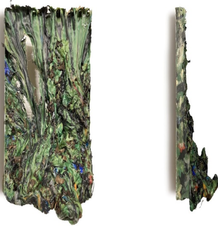
Figure 10: Allowing gravity to allow the hot plastic to sump and stretch in the mold. Source: (Author 2023)
