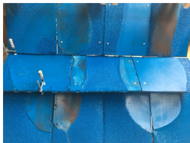
Figure 4: Detail of Polycarbonate panel assembly showing collage of imperfection characteristics created by top plate pressure application. Source: (Author 2022)
