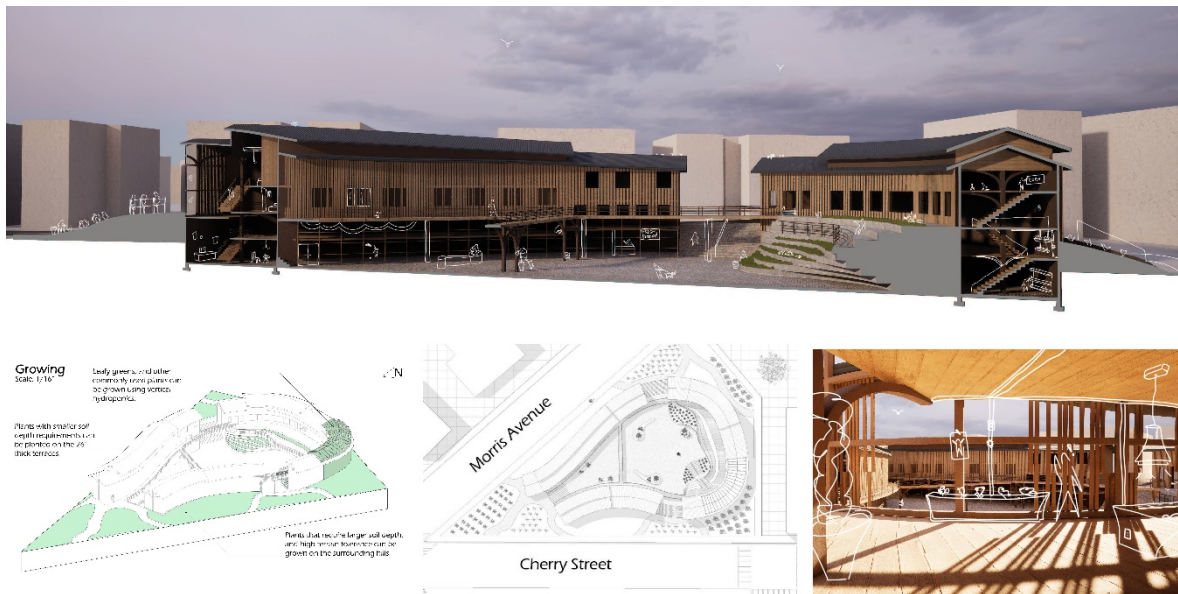
Figure 06: Images from Christian Garganta's project. Rendered section perspective (top), growing diagram (bottom left), site plan (bottom middle), and interior rendering (bottom right). Source: (Author 2023)
