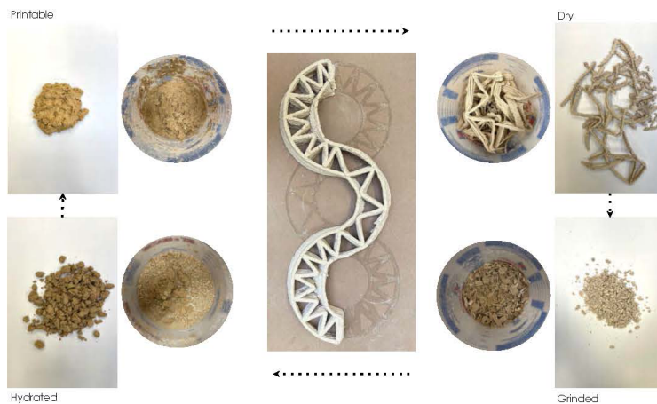
Figure 4: Material recycling process from bone dry to slurry. Source: (Created by the authors 2024)
