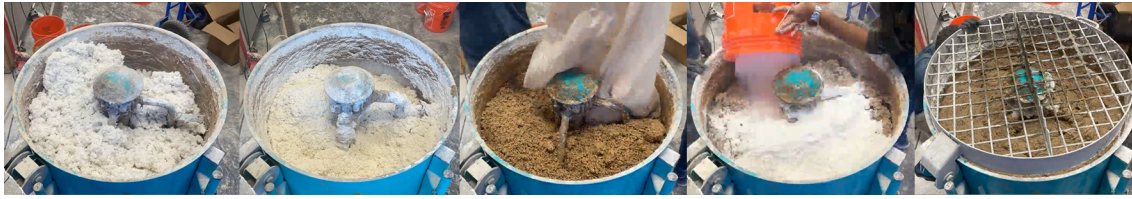
Figure 3: Material mixing process. Left to right: Paper pulp, saw-dust, hydrated mix of paper and saw-dust, dry mix of other ingredients, and final slurry. Source: (Created by the authors.)
