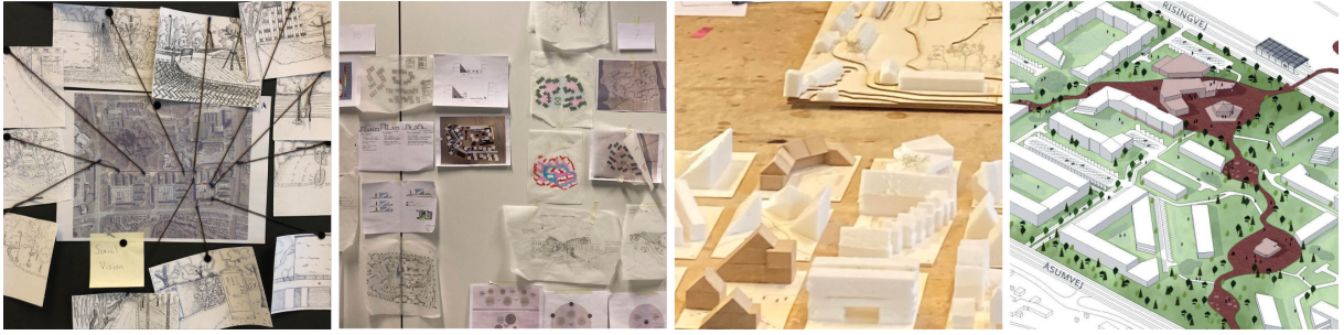
Figure 1: Glimpses into the collection of visual material used throughout the process of proposing design solutions on building scale. From left to right illustrating respectively elements from the analysis (maps with annotations), hand-drawn sketches, model exploration on building scale and graphic renderings of final designs. Source: own material (Berger and Olsen 2024)
