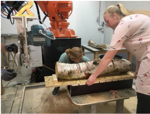
Figure 2: Student positioning log in front of an industrial robot with a bandsaw. Source: (Authors 2019)
