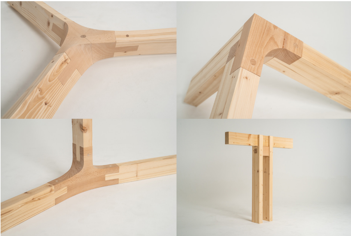
Figure 10: CNC-milled beech joints. Result of workshop 2. Source: (Various students and Authors 2020)
