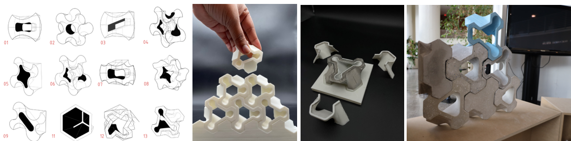
Figure 5. Project Re-Block. A series of topological interlocking geometries were explored (left); the selected interlocking geometry was 3D printed in PLA (middle); Final mold design (left). Design and drawings by Avinash Verma and Krishna Jayachandran. Source: (Author 2024)
