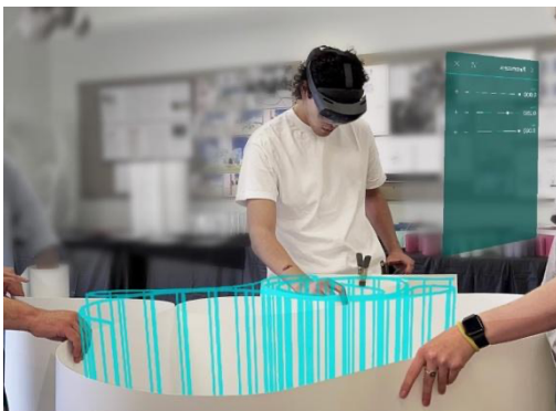
Figure 7: The 1:1 augmented prototype assembly process shows the geometrical overlay and the user interface. Source: (Author 2024)
