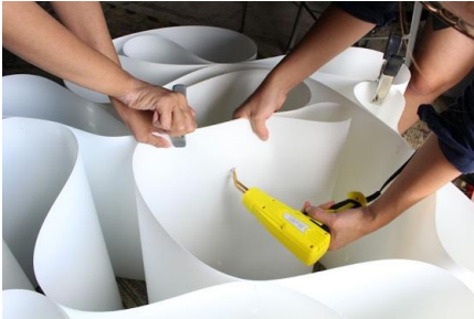
Figure 8: The W-shaped fusion welding tool and its application for the 1:1 prototype. Source: (Author 2024)
