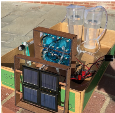
Figure 1: A demonstrator of using RPEMFC to store energy. Author: (Zhang and Azari 2025)
