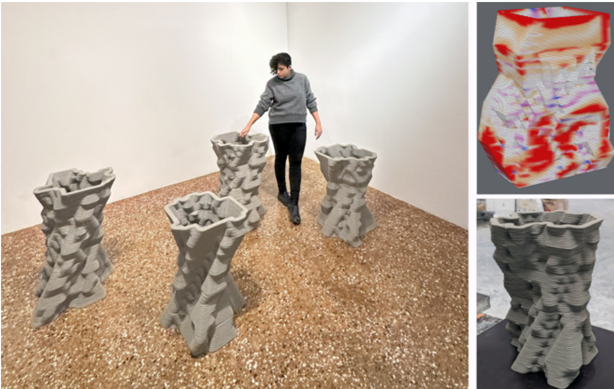
Figure 8: Left: Prototypes showcasing the voxel-based continuous robotic concrete 3D printing approach; right Finite Element Method analysis of the surface, guiding recursive voxelization for additional reinforcement where needed. Source: (Left: Authors, 2023–24. Design and research developed as part of the Design Computation (DCF) ARCH 5604 studio and Smart Materials ARCH 5303 course, led by S. Mostafavi, and the Urban Community Design (UCD) ARCH 5604 course, led by A. Mehan, at TTU in Spring 2023, exhibited at the ECC Venice Architecture Biennale. Right: Photos taken and produced by XtreeE, an industry collaborator on the project)
