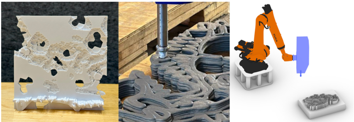
Figure 1: AI-Generated Printable Porosity: Left - Macro-scale cellular structure generated with AI; Middle - Continuous printing at varied heights; Right - Simulation diagram of the print. Source: (First and second Authors, 2022. Design, methods, and research developed as part of ARCH 5354 at TTU, led by S. Mostafavi. Team: Abel Gonzalez, Edgar Montejano, Cristian Solis, Matthew Stevens, Benjamin Varner)
