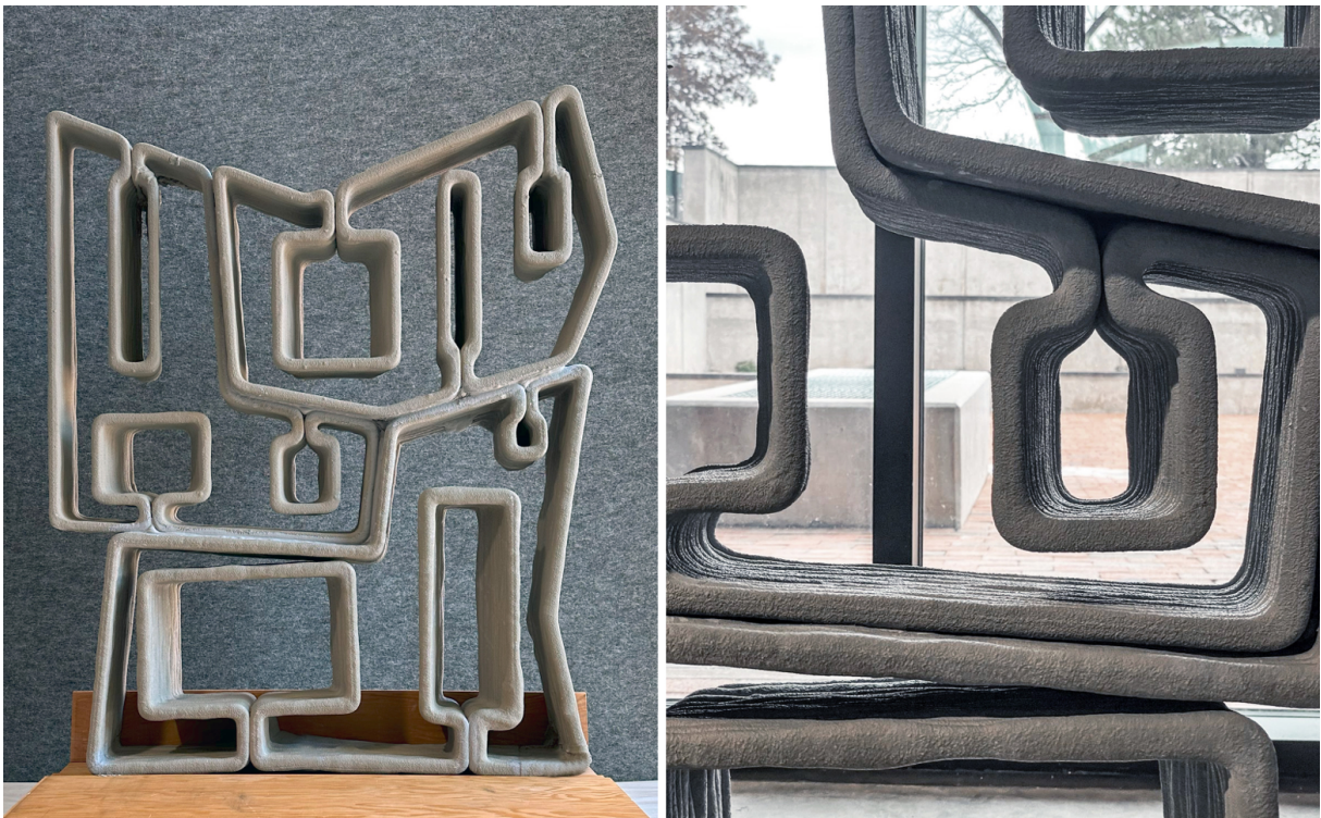
Figure 4: Left: A one-to-one prototype of the Concrete 3D-Printed Stacked Wall featuring three L- and V-shaped components; Right: a close-up view of the tapered niches. Source: (First Author, 2022. Design, methods, and research developed as part of ARCH 5354 at TTU, led by S. Mostafavi. Team: Elias Hernandez, Alexis Hunsucker, Zahra Khodabakhsh, Maria Guadalupe Martinez, Derek Williams)
