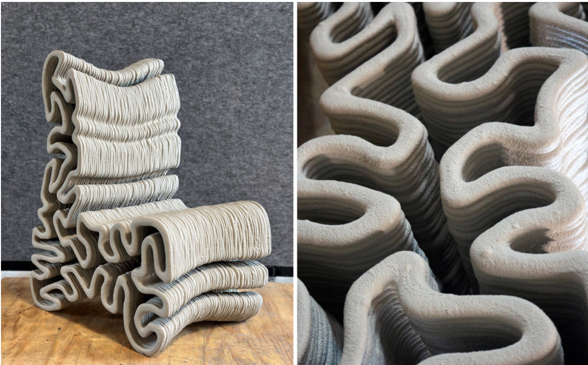
Figure 6: Left: One-to-one prototype of RC3DP Reaction-Diffusion Bench, Close-up of the continuous printed pattern. Source: (First Author, 2022. Design, methods, and research developed as part of ARCH 5354 at TTU, led by S. Mostafavi. Team: Luke Conrad, Saul Ortega, Judith Peralta Velazquez, Amanda Rich, Georgia Thomas)
