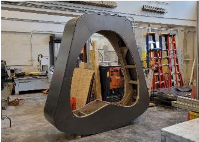
Figure 10: Rocking chair in progress fabrication photograph of wood framing and steel cladding. Source: (Dickey 2023)
